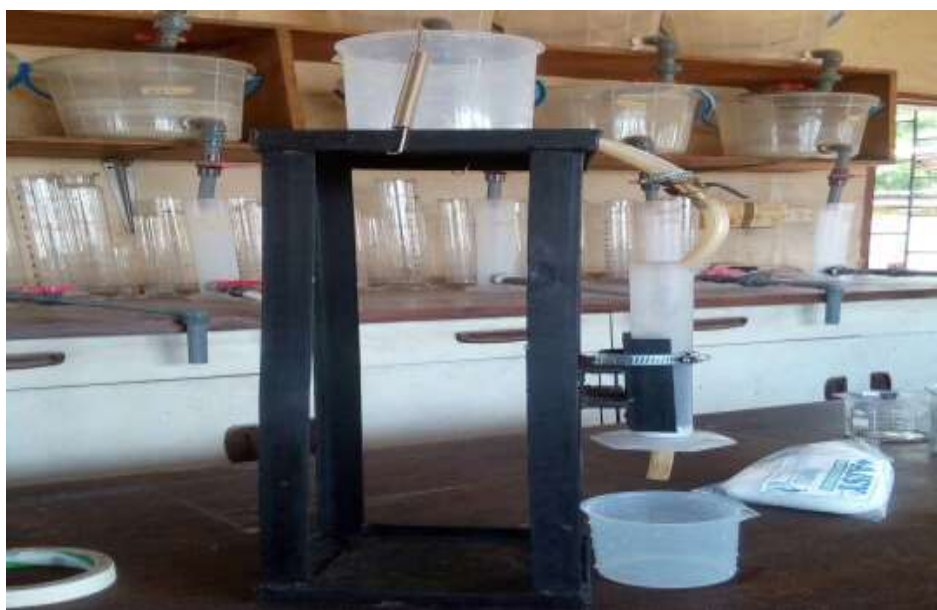
Figure 4: fixed bed column experimental set up
